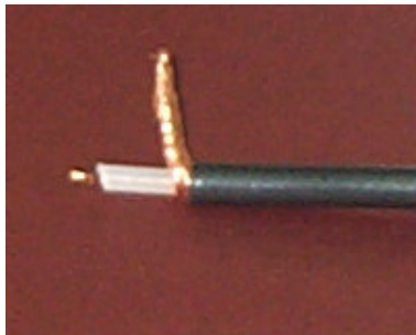
Figure 7: Stripped back sheath and twisted braid
